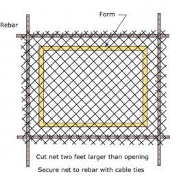
Pour-In-Place nets are used over stairway, elevator, and duct openings for passive fall protection, supplementing or replacing temporary floor covers. The high strength PSN rated nylon netting will absorb a dynamic load of 1300 lbs. When no longer required, the netting is simply cut away, allowing for continued construction. Standard and custom sized roll netting is available.
